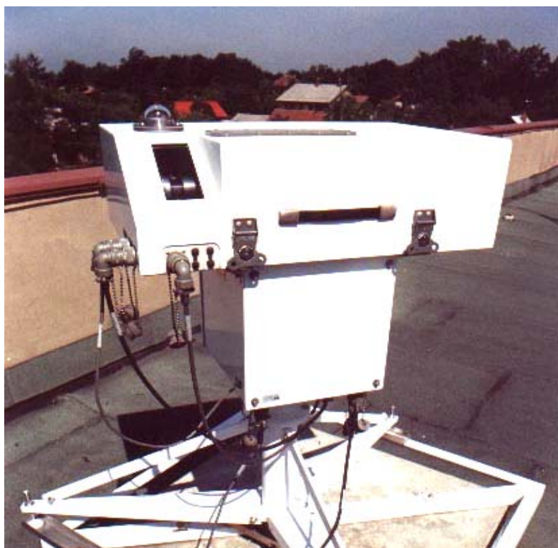
Figure 8. The Brewer MARK-IV spectrophotometer B098 operated at the Solar and Ozone Observatory in Hradec Králové
