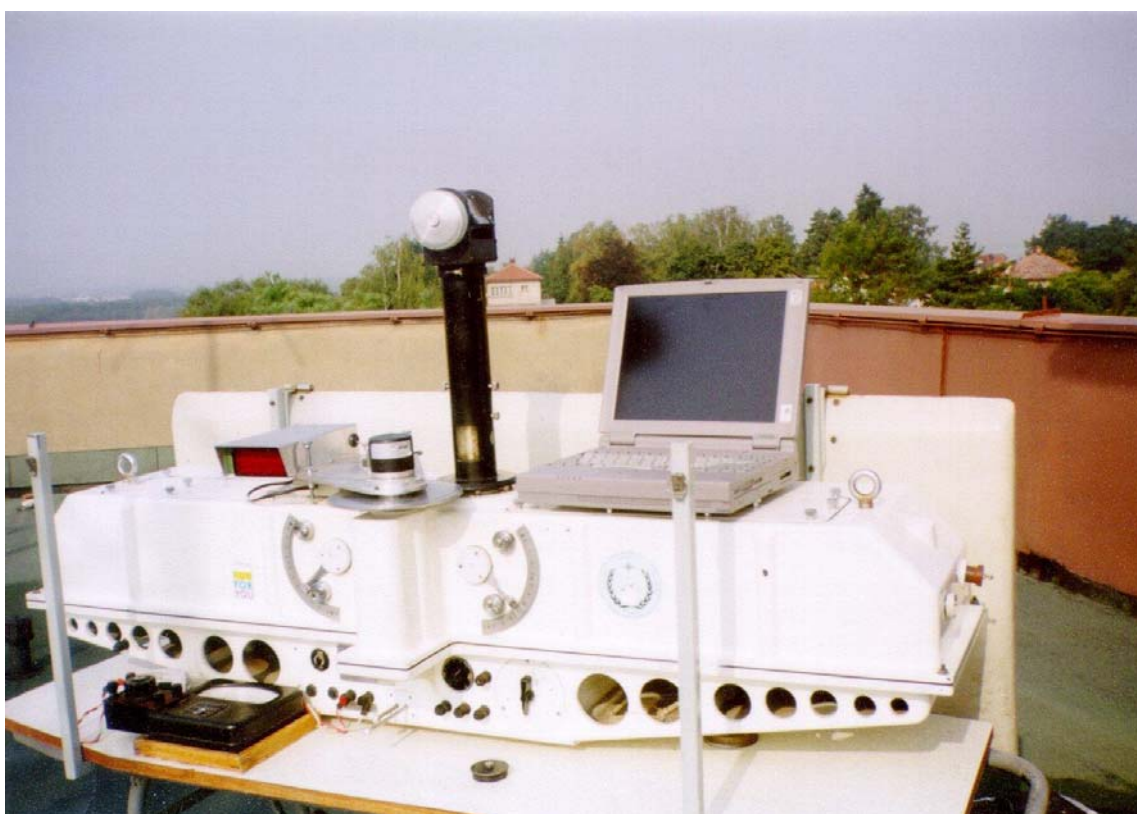
Figure 1. The Dobson ozone spectrophotometer D074 operated at the Solar and Ozone Observatory in Hradec Králové (SOO-HK) equipped with a semi-automated facility for data recording and processing of observations
